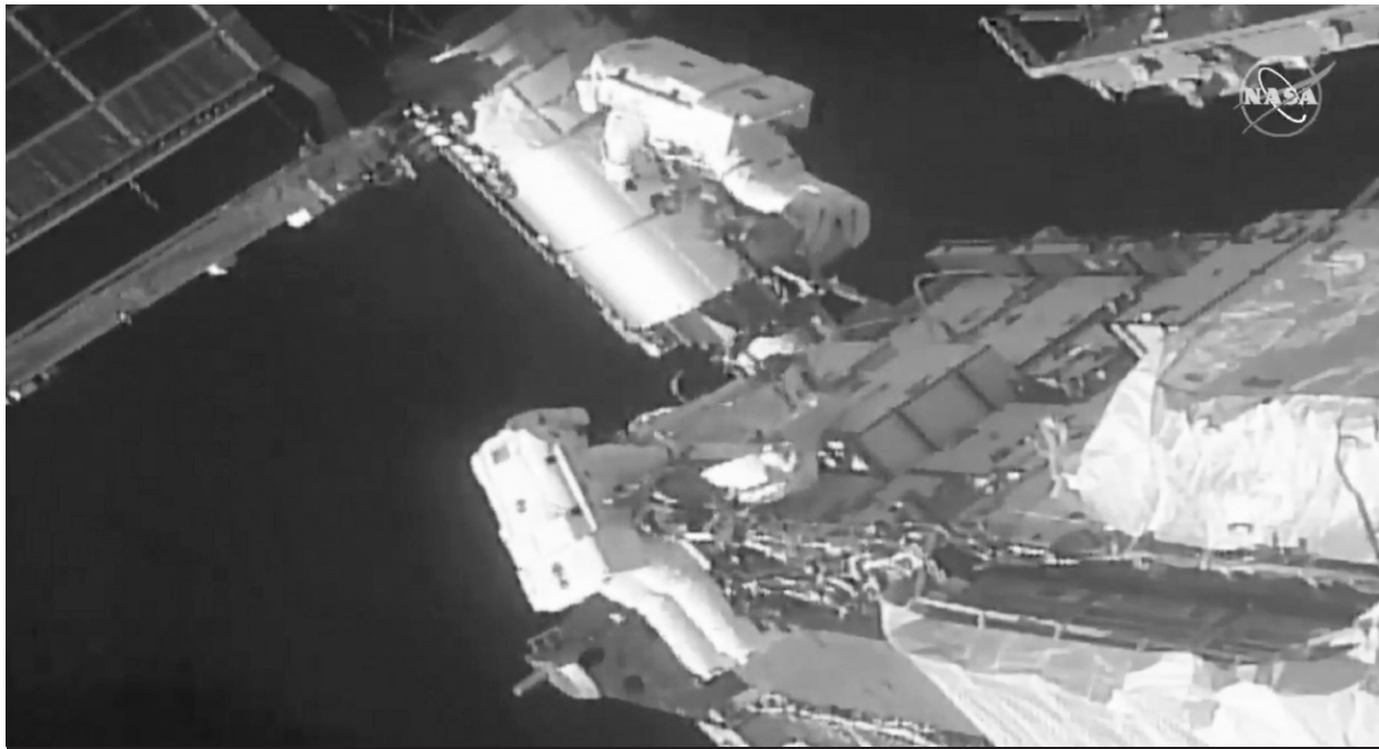
NASA astronauts Kate Rubins, top, and Victor Glover work outside the International Space Station Sunday, Feb. 28, 2021. The spacewalking astronauts ventured out Sunday to install support frames for new, high-efficiency solar panels arriving at the International Space Station later this year. (NASA via AP)
